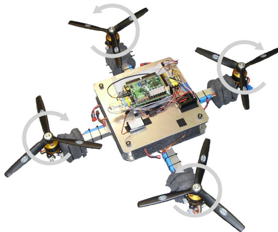
Figure 2.4: Balanced thrust resulting in a hovering platform
