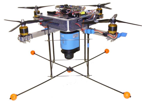
Figure 8.5: LADAR installed on the quadrotor
